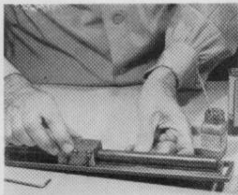
4. SLIDE BLOCKS should be lapped after reaming to assure smooth operation. Drill-rod track is coated with lapping compound. Block is stroked by hand
