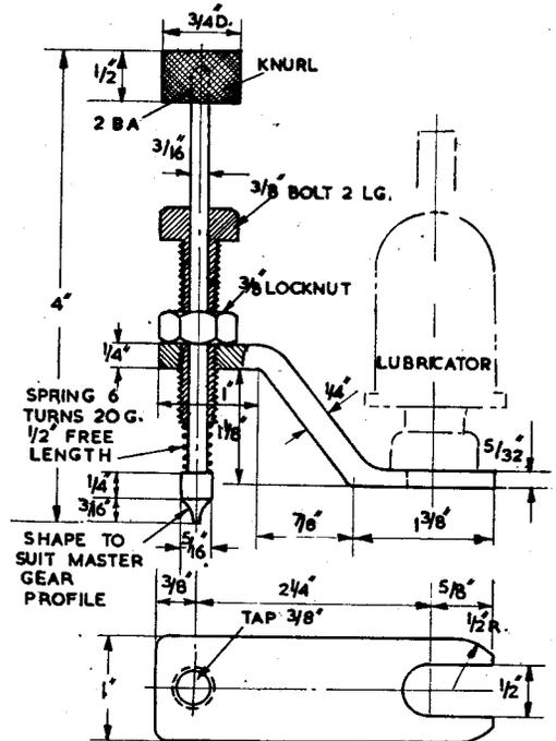
made a special divider by drilling as accurately as possible 3/32 in. dia. holes round the circumference of a brass disc. The disc was large enough to make small errors even smaller on the actual gear.
