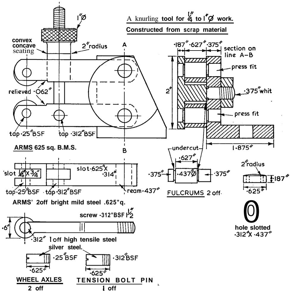
fulcrum pin had slots for a screwdriver in the plain end. I took care to arrange the threads of these so that any seizing effect from the pressure on the wheels would tighten the threads, assuming that the work would always be revolving top towards the operator.
