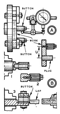
can be used direct The work is lightly clamped for truing, which is done with a lead hammer, or with a brass or copper drift and ordinary hammer. When the button is spinning truly, the work is fully clamped.
