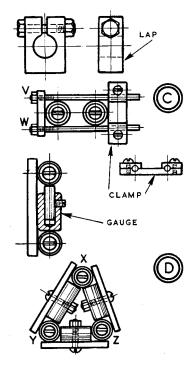
hardened, or cast steel ones which are hardened and tempered, can be lapped on the outside on a mandrel, 2, while the end can be lapped or ground with the button in a split holder, 3. This can be machined in the independent chuck. For lapping the outsides, a lap can be in brass or aluminium, adjusted by a bolt.
