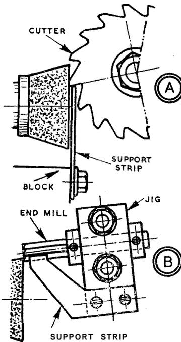
rotor or a wide roller mill, can be sharpened on lathe set-ups. With any spiral tooth cutter, either it or the grinding wheel must be traversed, while the cutter is kept down to the support strip-so that it turns slightly in grinding a tooth.
