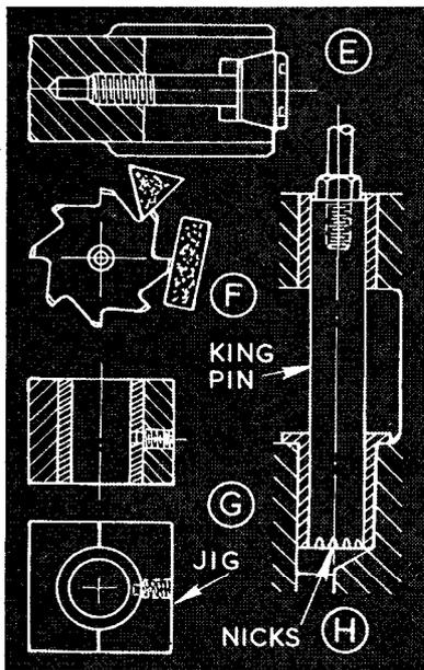
In all reaming, machining or hand, rotation is very slow and ample power is essential. In hand work, either the component is held in the vice and the reamer turned with a substantial tap wrench, or the reamer is held and the component turned-when it is a size and shape permitting proper leverage.
