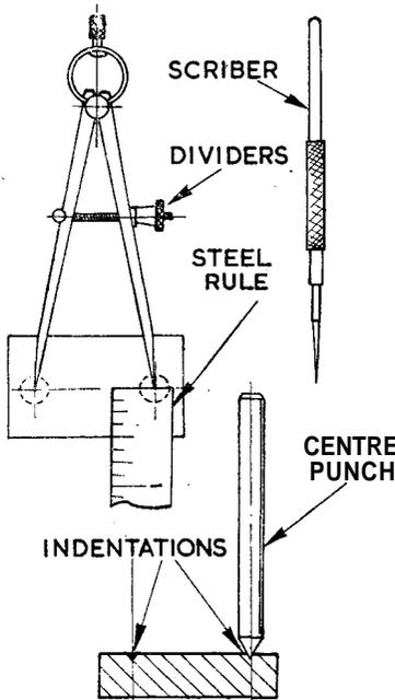
Fig. 1.—Preparing the work for drilling
