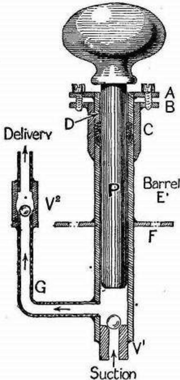
FIG. 109.—Vertical section of force pump.
