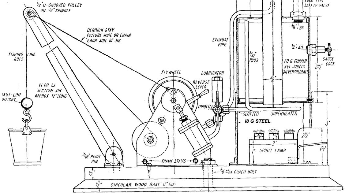
General arrangement and part plan for a simple steam crane
