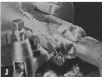
**Cylinder covers** are turned from  $1\frac{1}{2}$ " brass rod. Inside face of upper and lower covers are turned to a snap fit in cylinder bore, using cylinder as gauge. Then they are cut off, reversed in the chuck and finished. Piston-rod packing-gland hole should be drilled and tapped in lower cover before cutting off.
