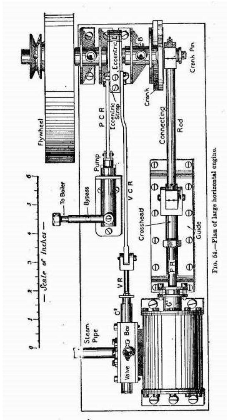
FIG. 54.—Plan of large horizontal engine.
