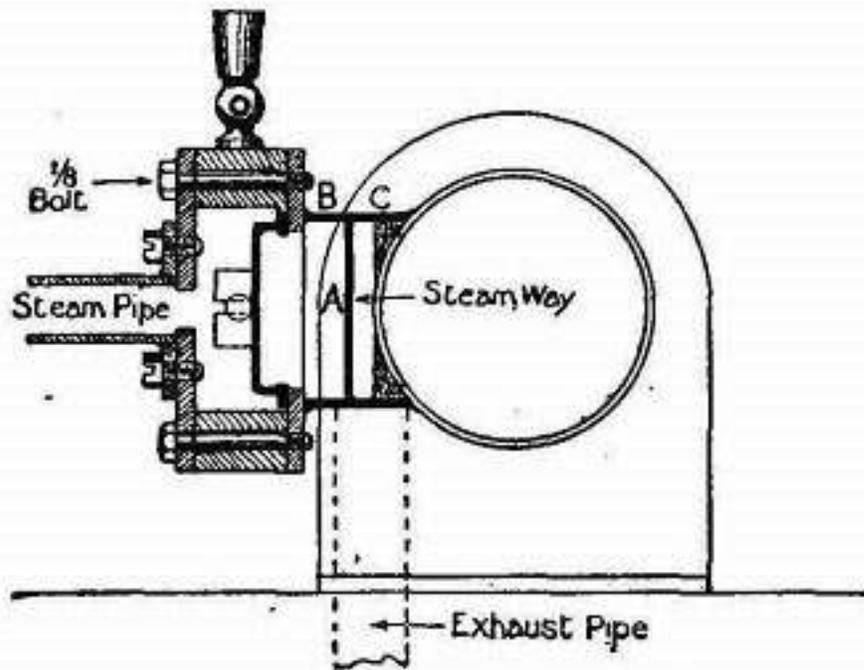
FIG. 62.—Cross section of cylinder and valve chest.
