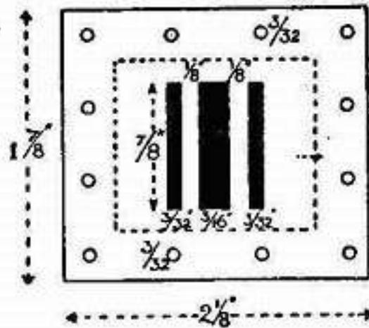
**FIG. 59.**—Valve plate.
