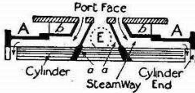
FIG. 61.—Valve plate and steam ways in section.
